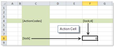
The lock and unlock tags support one optional parameter, to define a target size for the lock or unlock operation. Within an action tag pair, one tag can have the optional parameter, and the other tag must be just [Lock] or just [Unlock].
